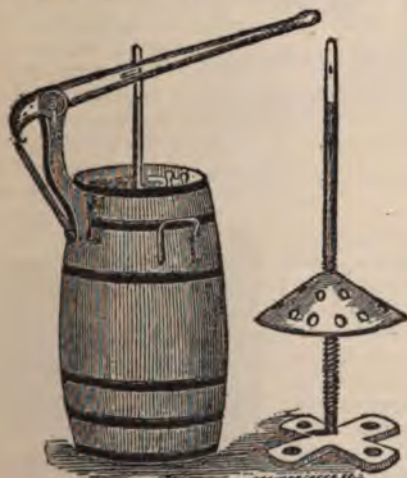
Fig. 194. An adjustable dash churn.
